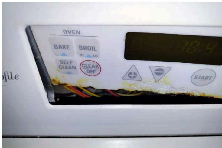
[PHOTO: Complete separation from stove body with exposed internal wiring and rust-colored staining]
