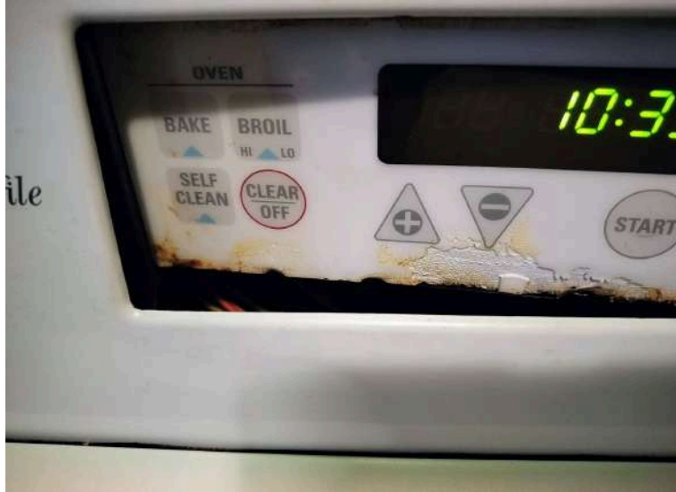
[PHOTO: Control panel with digital display showing separation with brownish-yellow discoloration]
